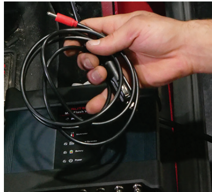
7. Connect 12-volt adapter plug to VCI/VCMI
