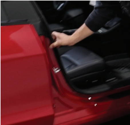
1. Open passenger door and detach the rubber molding around the door frame.
