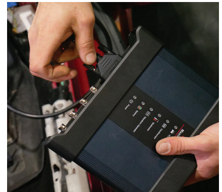
6. Connect cable to VCI/VCMI
