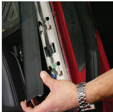
3. Remove trim panel by carefully prying up and pulling back towards door.
