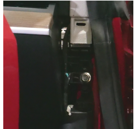
2. Detach small black panel adjacent to dash. Remove clip.
