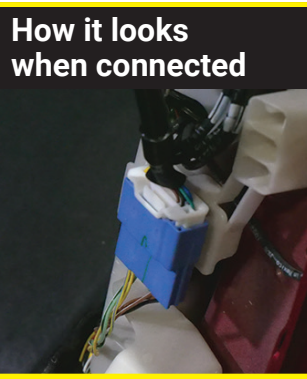
5. Plug the TCAN001 cable into the Blue connector
