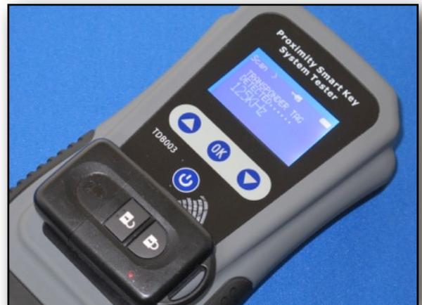
THE TDB003 WILL INDICATE THE TRANSPONDER HAS BEEN DETECTED AND THE FREQUENCY THE TRANSPONDER OPERATES ON.
