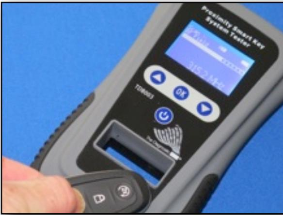
THE TDB003 WILL DISPLAY THE FREQUENCY OF THE REMOTE CONTROL AND ALSO THE SIGNAL LEVEL ON THE BAR GRAPH.
