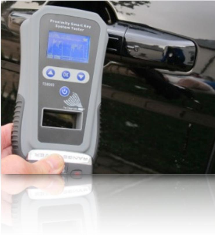
IN OSCILLOSCOPE MODE THE SIGNAL LEVEL OF THE SMART/ PROXIMITY KEY CAN BE VIEWED AND COMPARED.
