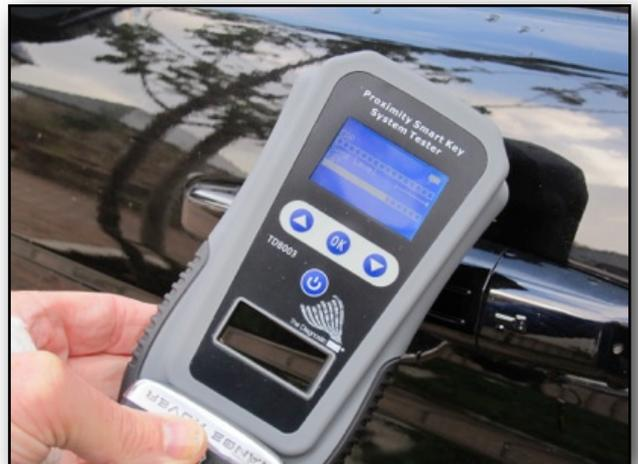
OPERATE THE PROXIMITY SYSTEM BY TOUCHING THE SENSOR, BUTTON OR OPENING THE DOOR.
