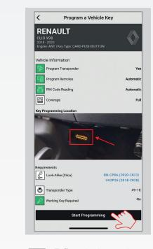
Follow the instructions in MYKEYS Pro and connect the Smart Pro Mini to the vehicle OBD using the cable provided.
