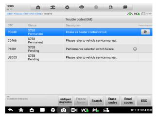
Figure 4-24 Sample DTC & FFD Screen
