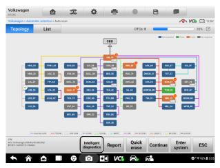
Figure 5-2 Intelligent Diagnostics Button (Topology Screen)
