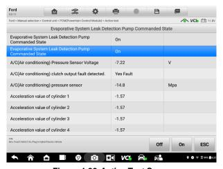
Figure 4-22 Active Test Screen
