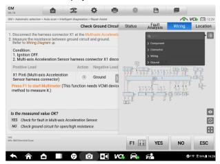
Figure 5-18 Repair Assist Screen 5
