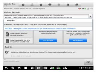
Figure 5-11 Vehicle System and Detected DTC(s) Screen
