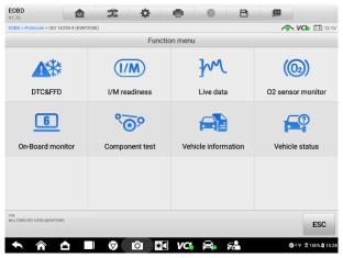
Figure 4-23 Sample OBDII Diagnostic Menu
