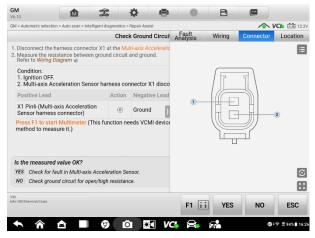
Figure 5-20 Repair Assist Screen 7
