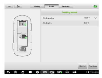
Figure 9-7 Starter Test Results Screen
