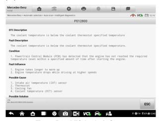
Figure 5-13 DTC Analysis Screen
