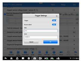
Figure 4-21 Trigger Settings Screen
