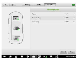
Figure 9-8 Generator Test Results Screen
