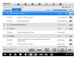
Figure 5-5 Enter System Button (List Screen)
