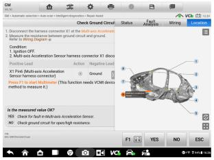
Figure 5-19 Repair Assist Screen 6
