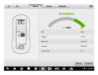
Figure 9-6 Battery Test Results Screen
