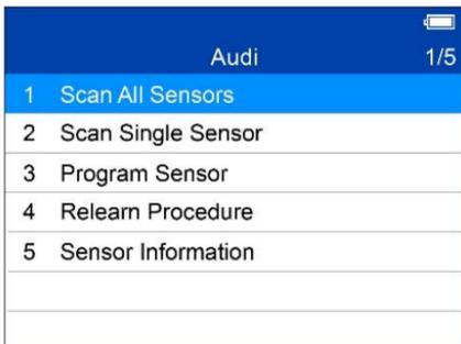
Select Scan All Sensors. Hold the tool close to the sensor or close to the tire sidewall right above the sensor.
